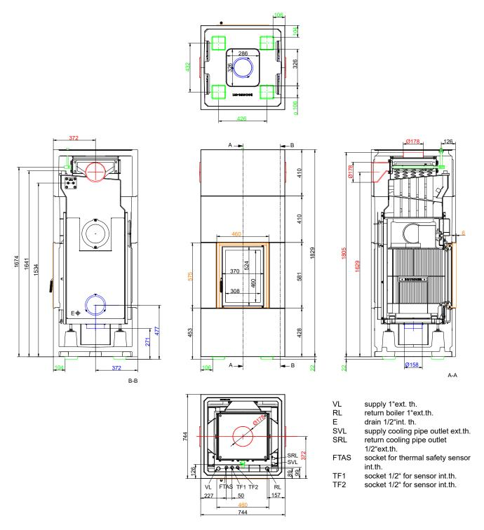
We suggest for CAD planning Palette CAD. Permanent updated drawings: www.brunner.de Frames/ flue gas outlet connection/ combustion air supply connection/ front variants/ support bearing are marked in color.
